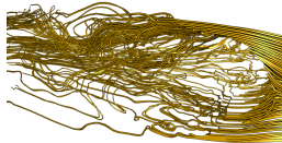
(a) 500 opaque path lines with 500 segments each, depth-dependent halos and 4x MSAA at 55fps.
