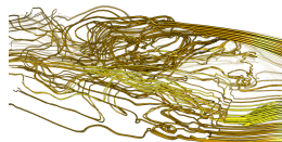
(d) Fragment linked lists with screen contribution blending and brushing. Achieves 13fps at 4x MSAA.
