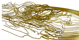
(c) Fragment linked lists with screen contribution blending. Achieves 16fps at 4x MSAA.
