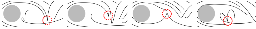
Fig. 6 Path lines in the flow behind a cylinder have been seeded using Algorithm 1, but without excluding the areas around cusp seeding lines. While the result is free of (self-)intersections, some path lines exhibit cusps or cusp-like shapes (highlighted by red circles).
