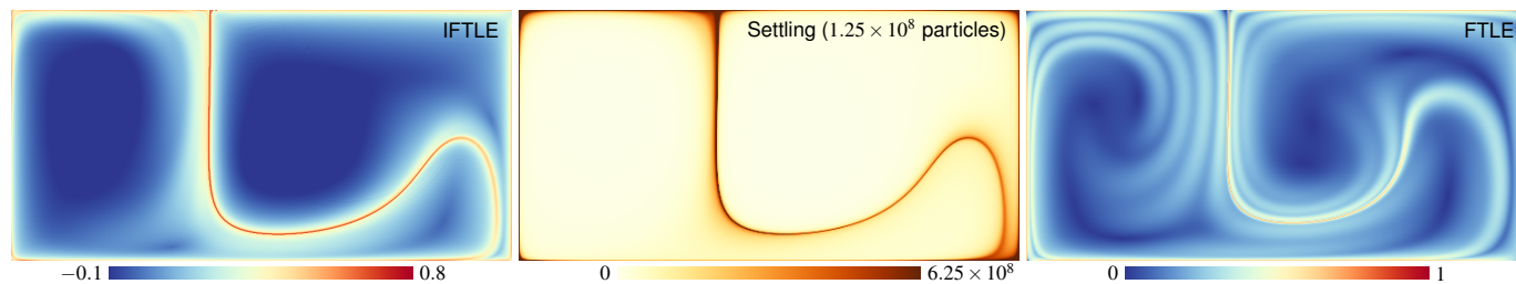
Fig. 1: Backward FTLE of inertial particles as computed from influence curves [28] (left) correlates with preferential particle settling (center). In previous work, particle settling has been analyzed by backward FTLE on tracer particles [66] (right), which shows resemblance but is not as accurate. Here, in the DOUBLE GYRE with d_p = 200 \mu\text{m} , start time t_0 = 0 and integration duration \tau = 9 .
