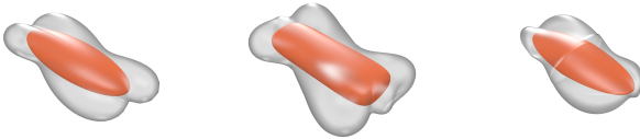
Figure 9: Glyphs for uncertain tensor with \bar{\mathbf{S}} = \begin{pmatrix} 1 & 0.2 & 0.1 \\ 0.2 & 0.4 & 0.03 \\ 0.1 & 0.03 & 0.2 \end{pmatrix} and \mathbf{C} = 10^{-3} \cdot \begin{pmatrix} 103 & 69 & 69 & 0 & 0 & 0 \\ 69 & 66 & 36 & 0 & 0 & 0 \\ 69 & 36 & 66 & 0 & 0 & 0 \\ 0 & 0 & 0 & 300 & 0 & 0 \\ 0 & 0 & 0 & 0 & 6 & 0 \\ 0 & 0 & 0 & 0 & 0 & 200 \end{pmatrix} .
