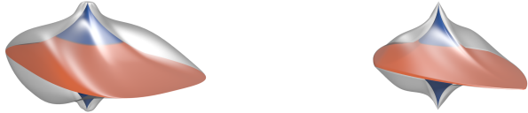
Figure 8: Glyphs for uncertain tensor with indefinite mean \mathbf{v}(\bar{\mathbf{S}}) = (1, 0.6, -0.5, 0, 0, 0)^T and \mathbf{C} = \text{diag}(0, 0.65, 0.03, 0, 0, 0) . The tensor varies in one principal direction. Left: superquadric glyph with u(G) \approx 1.5 \cdot 10^{-4} . Right: glyph by [GRT17a] with u(G) \approx 3 \cdot 10^{-6} . (There exists no ellipsoid glyphs in the indefinite case.)
